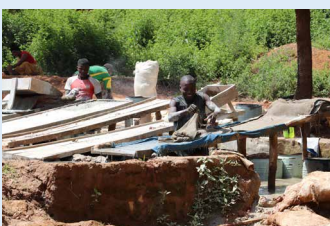
Figure 4: ASGM production steps: concentration and mercury amalgamation at ASGM site in Kenya
