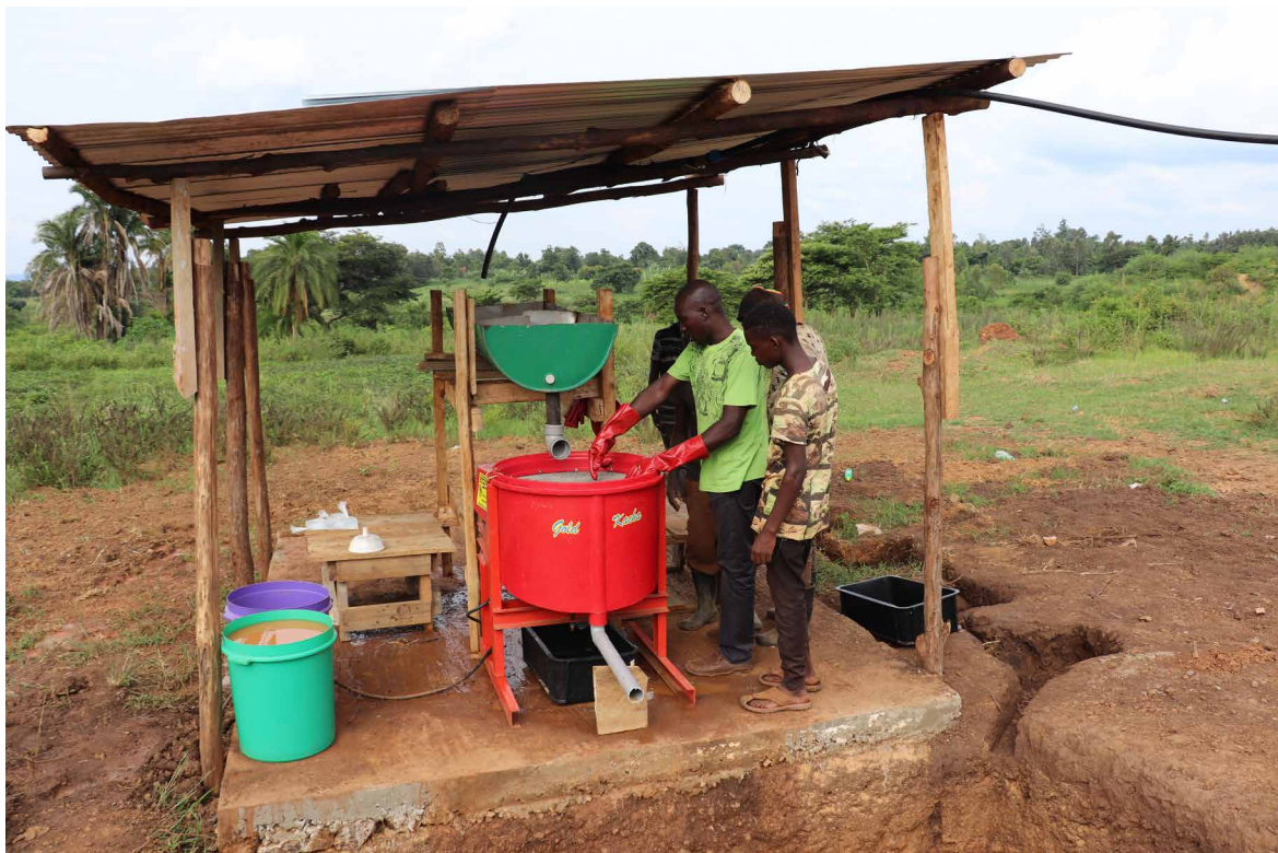
Figure 12: Gold Kacha without a sluice box located in Busia, Uganda, installed and operated by TIF throughout 2019 and 2020
