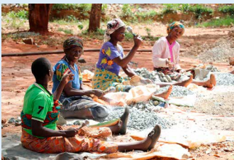
Figure 3: ASGM production steps: ore crushing and milling at ASGM site in Tanzania
