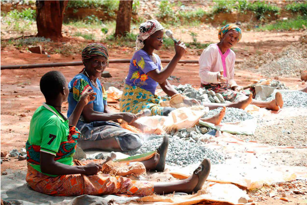
Initial hammering of the gold ore into smaller pieces before mechanical crushing
