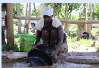
Figure 4: ASGM production steps: concentration and mercury amalgamation at ASGM site in Kenya
