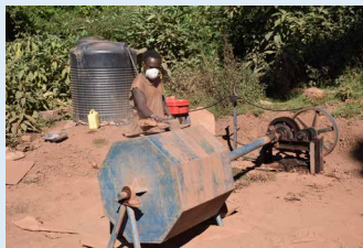
Figure 3: ASGM production steps: ore crushing and milling at ASGM site in Tanzania
