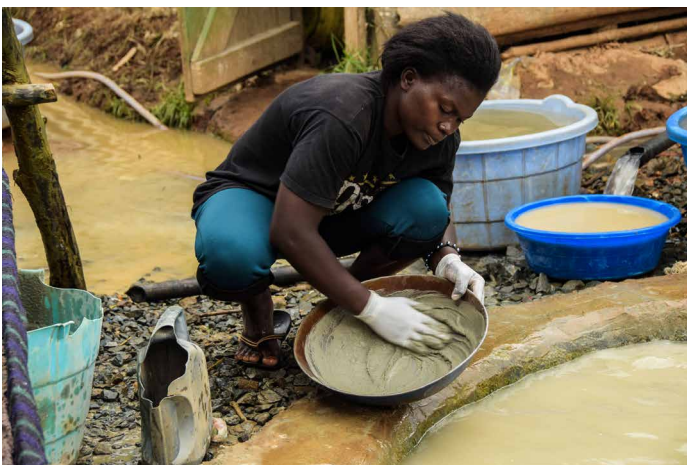
Figure 7: A mine worker wearing latex gloves while washing gold into a washing pond
