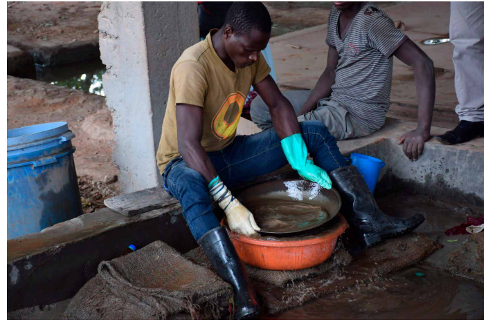
Figure 8.2: A miner in Tanzania demonstrates the panning process with makeshift gloves
