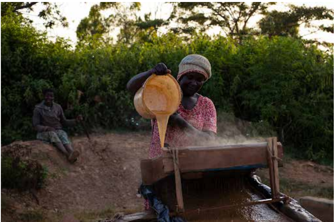
Sluicing, the first concentrating process to trap gold on the inclined ore before the panning method in artisanal mining
